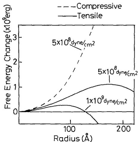
FIG. 8. Change in the free energy associated with void formation in an equiaxially stressed aluminum lattice.
