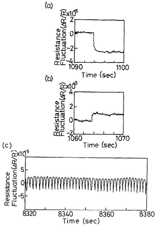
FIG. 3. Three types of ACRs: (a) downward step, (b) upward step, (c) oscillations. Time was counted from the beginning of the EM test. Temperature was 192 °C, and the current density was  $4 \times 10^6$  A/cm<sup>2</sup>. The length of the interconnection was 1350  $\mu$ m.
