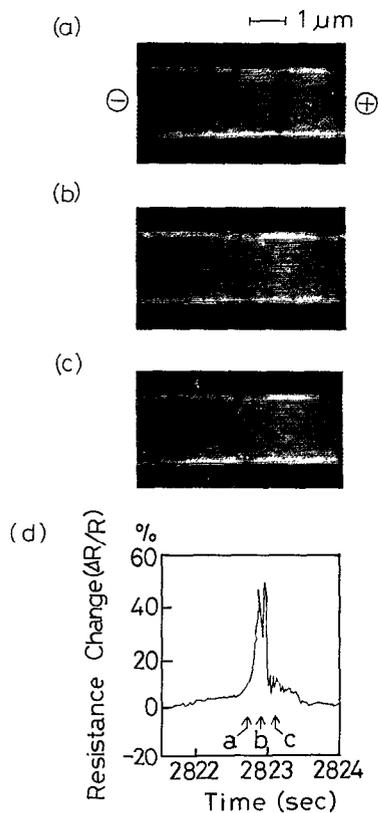
FIG. 6. Observation of rapid void annihilation and subsequent formation by SEM (a)–(c) and corresponding resistance change (d). Arrows indicate times when photographs were taken. Temperature was  $200^\circ\text{C}$ , and the current density was  $1.1 \times 10^7 \text{ A/cm}^2$ . The length of the interconnection was  $100 \mu\text{m}$ .
