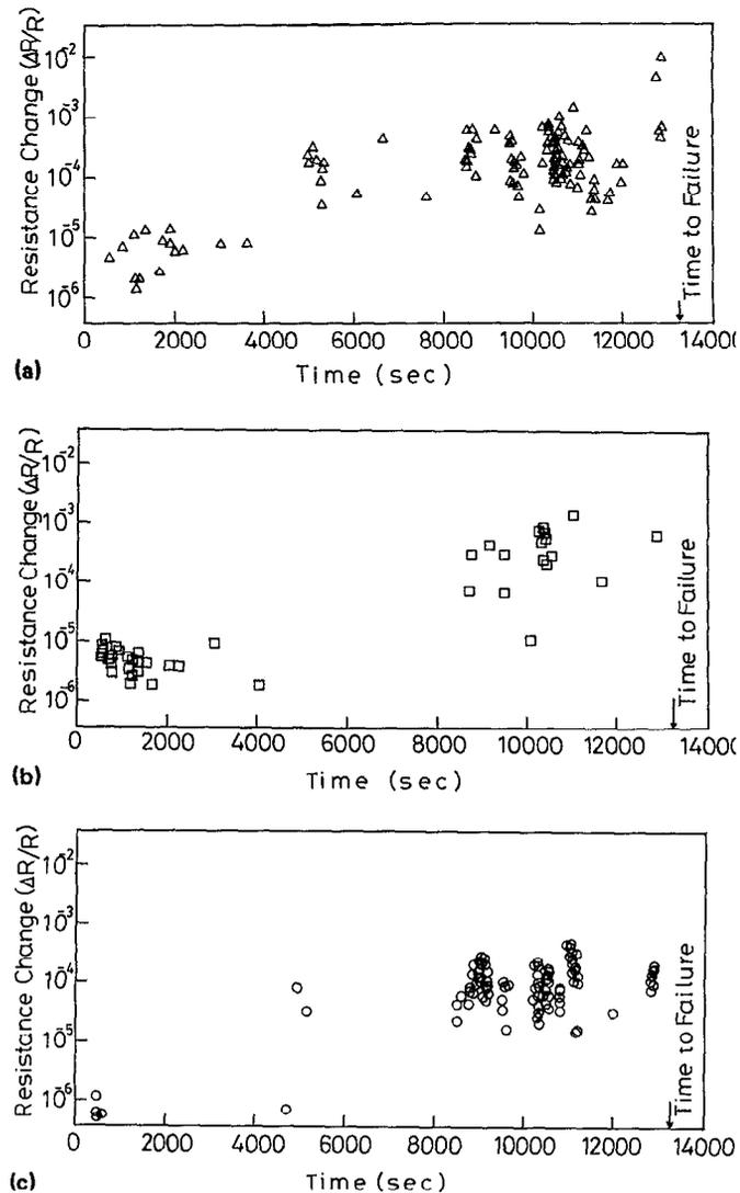
FIG. 4. Occurrences of ACRs through the EM test: (a) downward steps, (b) upward steps, (c) oscillations. Each circle corresponds to one period of oscillation in (c). Temperature was 192 °C, and the current density was  $4 \times 10^6$  A/cm<sup>2</sup>. The length of the interconnection was 1350  $\mu$ m.
