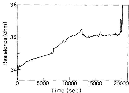
FIG. 2. Resistance change of aluminum interconnection during an EM accelerating test. Current density was  $4 \times 10^6 \text{ A/cm}^2$ , temperature was 250 °C. The length of interconnection was 1350  $\mu\text{m}$ .
