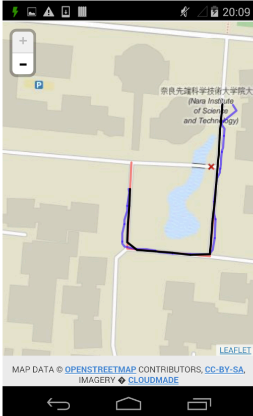
Figure 4: Screenshot of our application, which displays recommended route (red line), original trajectory (blue line), estimated evacuation route (black line), and blocked road segment (red cross).
